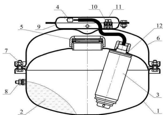
4.2 After receipt of an electrical impulse to the electrical output switch 4GSP 3 (Figure 1,2), the gas generator is activated and generates a cold gas that puts the interior of the container under pressure. As soon as the necessary pressure is present, the membrane opens 6 and the extinguishing powder comes out of the module through the atomizer 5.
